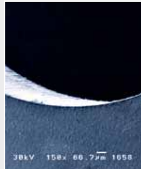
Precise cuts in sensitive materials (aluminum nitride).
